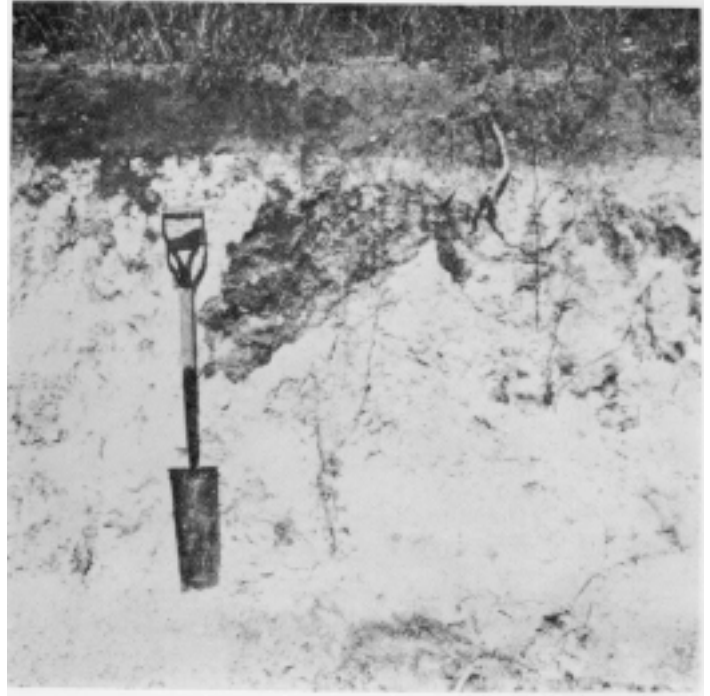
Figure 9.—Profile of Brackett clay loam, 1 to 5 percent slopes, showing roots in chalky underlying material.
