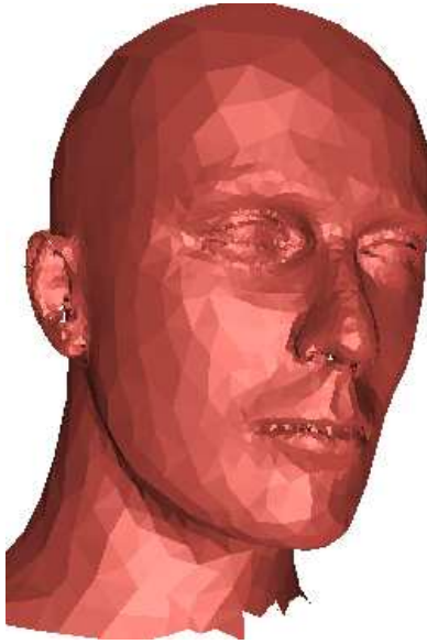
Figure 3.3: A set of candidate triangles. There are some holes in undersampled areas such as ears and nose and the boundary around the neck.
