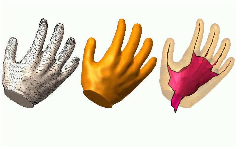
Figure 3.5: Samples from laser range scanner, the power crust, and the power shape
